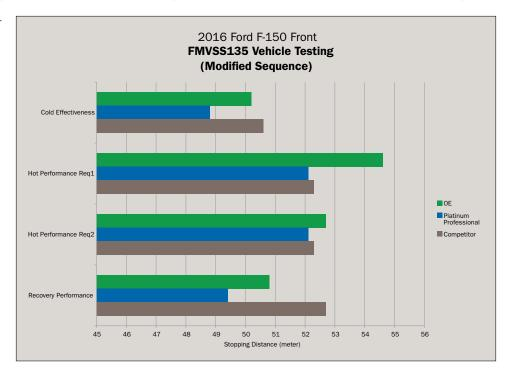
**Break-in** — Our revolutionary burnishing compound allows for proper break-in of pads and rotors. Take a look at how Platinum Professional improves stopping power from the first stop:
