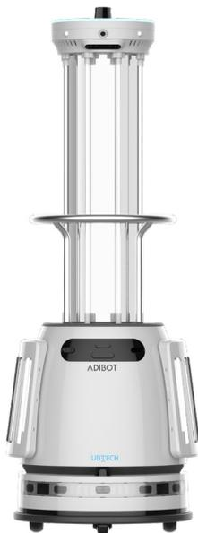
ADIBOT A Autonomous UV-C Disinfection Robot
