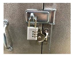
Our team wanted to have a locking mechanism to make sure the device couldn't be opened during operation and therefore students/staff could not be exposed to the UV-C light while the AIRrow 5000 is in operation.
