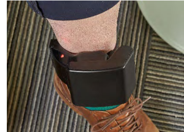
Figure 55. LOC8 XT Charging The LOC8 XT is charged by a wireless charger, allowing clients to easily maintain a charged device.
