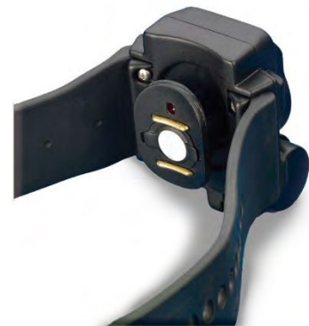
Figure 74. Alcohol Detection Sensor The Alcohol Detection Module (ADM) samples the alcohol content of the client's perspiration to determine the client's TAC level.
