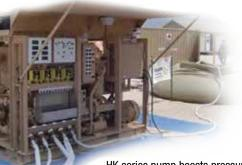
HK series pump boosts pressure a on 1500 ROWPU system
