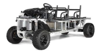
To prevent rust and ensure long life, look for vehicles built on rustproof, corrosion-resistant aluminum frames (shown above).
