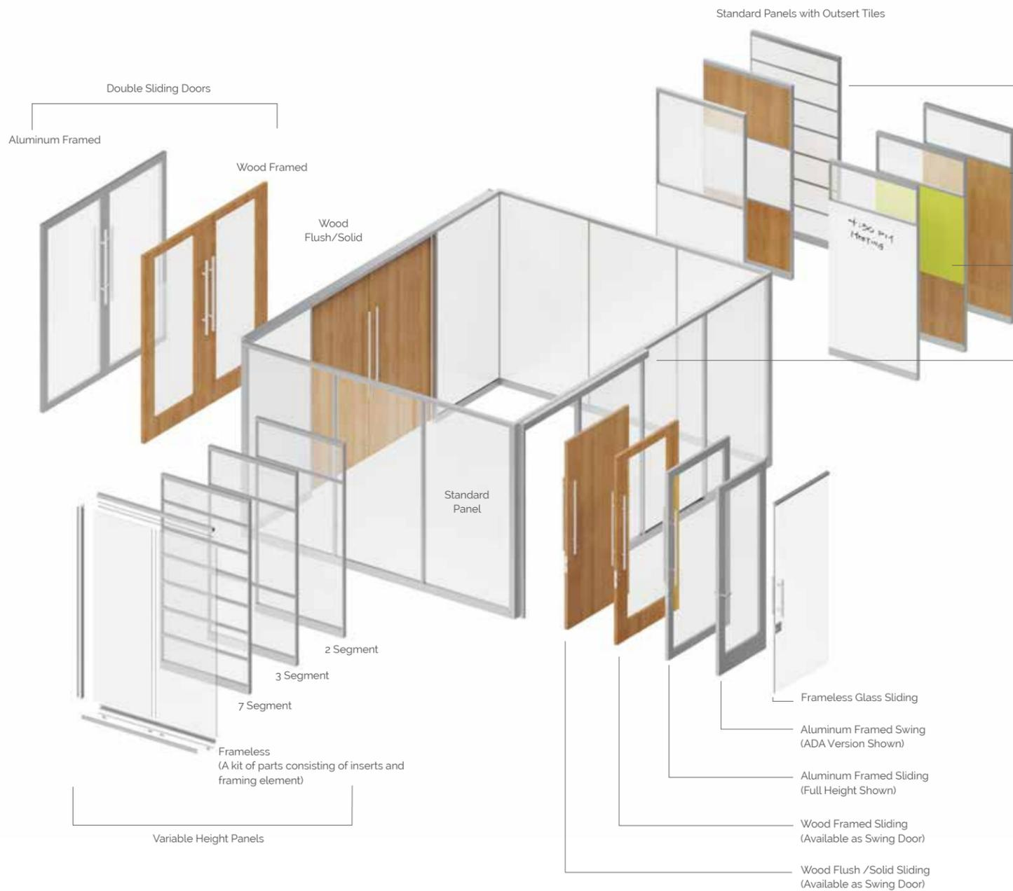
PANEL SEGMENTATION allows up to 7 Tiles of identical or varied materials on each side of the panel. Outsert and Insert Tiles can blend for maximum aesthetic and functional versatility. Different tile configurations can be specified for each side of a panel.
