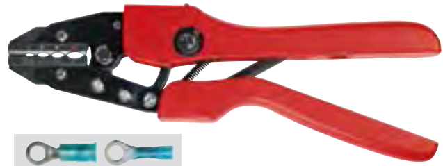
Ratchet Crimping Tool 22–8 GA Part No: RT822 Designed for heat shrink terminals. Four crimp nests: 8 AWG, 12–10 AWG, 16–14 AWG, 22–18 AWG. Ensures uniform crimp termination regardless of user. See page 532 for additional dies.
