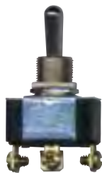
Part No: TSW22 Type: Single Pole/Double Throw (Mom. On/Off/ Mom. On) Number of Contacts: 3 Terminal Type: Screw
