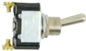
Part No: TSW20 Type: Single Pole/Single Throw (Momentary On/Off) Number of Contacts: 2 Terminal Type: Screw
