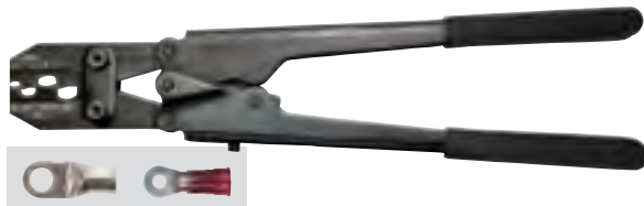
Compression Crimp Tool Part No: RC6220 For insulated and non-insulated lugs, 8–2 GA, 4 crimp nests.
