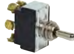
Part No: TSW4 Type: Double Pole/Double Throw (Mom. On/Off/ Mom. On) Number of Contacts: 6 Terminal Type: Screw
