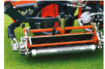
Unique swing out center cutting unit
