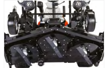
Low maintenance, direct drive hydraulic decks
