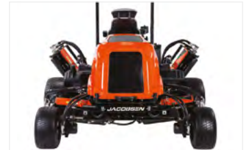
Wide stance rear axle for excellent stability and aftercut appearance
