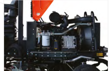
50.2 HP (37.4 kW) diesel Kubota® engine
