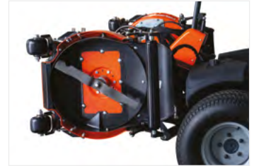
Vertical lift on outside decks for maneuverability
