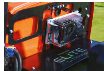
ELITE™ lithium battery & on-board high frequency 18 amp, 48V DC output, 85 - 265V AC 45 - 65 Hz input
