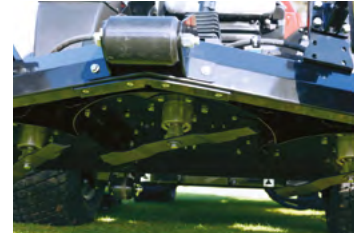
Low maintenance, direct drive hydraulic decks
