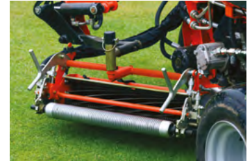
Unique swing out center cutting unit for ease of service
