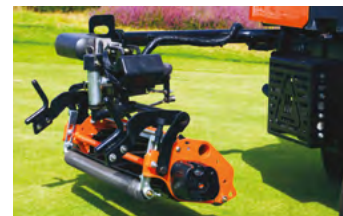
Easy access swing-out centre cutting unit
