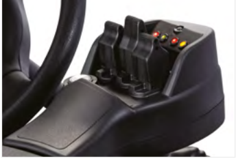
Fingertip lift / lower cutting unit controls
