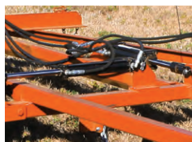
The STH2024 features a hydraulic lift for raising and lowering the harrow teeth.
