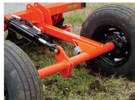
Optional hitch is self-leveling for pulling implements behind the Aerator.
