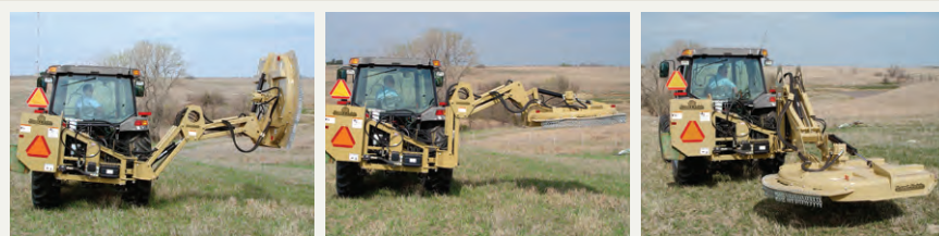
Hydraulic breakaway feature pivots arm backward to avoid obstacles and protect cutter arm. Hydraulically pivots back into place.
