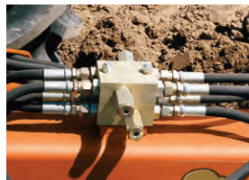
Optional cushion valve on the RBT45 protects cylinders and blade components during extreme impacts.
