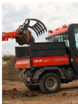
30" Jaw opening and open back for good visibility from tractor seat.
