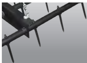
Teeth on both STH models are diamond shaped, 8-1/2" forged with hardened tip.
