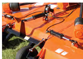
Dual leveling rods enable the cutter to pull equally on the rear axle during travel over rough terrain.
