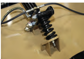
Center spring on the cylinder cushions load on drawbar.
