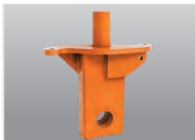
Pivot weldment features a 1" thick plate steel turntable, 3/4" thick tilt pivot bushing and a 4" solid kingpin.
