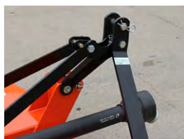
Cast floating top link follows ground undulations.
