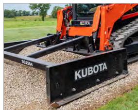
Full length, heavy-duty skid shoes are reversible and replaceable.
