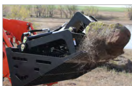
Grade 80 steel tine material with front gusseted tine tips.
