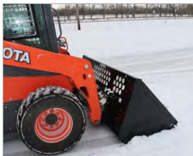
Cut out backplate provides increased visibility from the operator seat.
