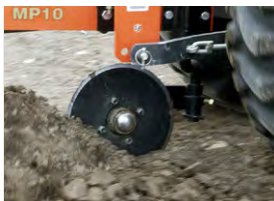
The optional coulters allow for a smoother furrow edge and help reduce slightly the drag on the moldboard.
