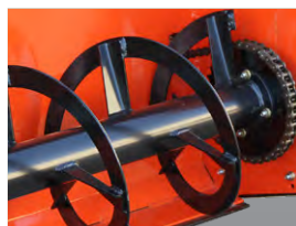
Augers are 3/8" x 2-1/2" with 14" or 16" diameter, and are protected by a shear-bolt.
