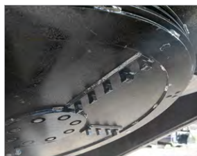
Replaceable carbide teeth on bottom of blade carrier.
