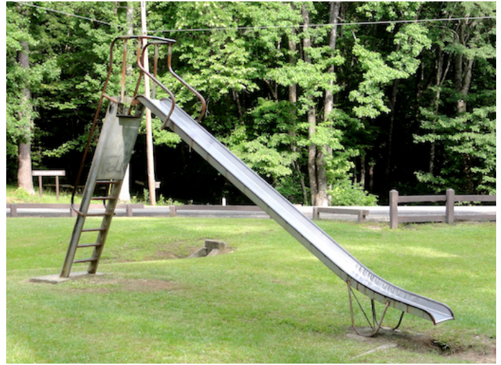
In addition to having unacceptable surfacing under it, this metal slide may become superheated on excessively hot days.
