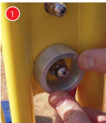
Gauges are used to test the compliance of all projections. This projection is in compliance because it does not extend beyond the face of the gauge.
