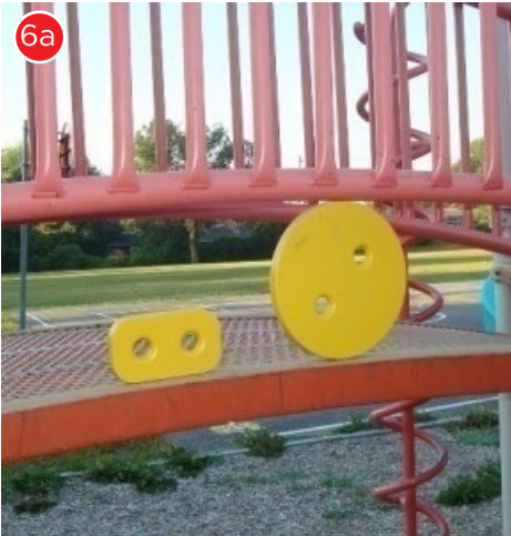
This photo shows the use of entrapment templates as opposed to the three dimensional probes.
