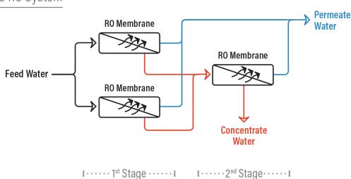
In a **Reverse Osmosis System** an array describes the physical arrangement of the pressure vessels in a 2 stage system. Pressure vessels contain RO membranes (usually from 1 to 6 RO membranes are in a pressure vessel). Each stage can have a certain amount of pressure vessels with RO membranes. The reject of each stage then becomes the feed stream for the
