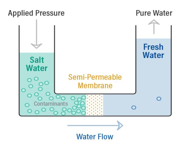
Reverse Osmosis works by using a high pressure pump to increase the pressure on the salt side of the RO and force the water across the semipermeable RO membrane, leaving almost all (around 95% to 99%) of dissolved salts behind in the reject stream. The amount of pressure required depends on the salt concentration of the feed water. The more concentrated the feed water, the more pressure is required to overcome the osmotic pressure.
