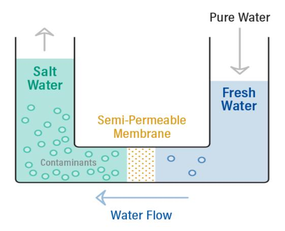
A **semi-permeable membrane** is a membrane that will allow some atoms or molecules to pass but not others. A simple example is a screen door. It allows air molecules to pass through but not pests or anything larger than the holes in the screen door. Another example is Gore-tex clothing fabric that contains an extremely thin plastic film into which billions of small pores have been cut. The pores are big enough to let water vapor through, but small enough to prevent liquid water from passing.
