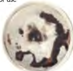
Mold covers the control sample completely
