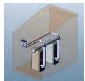
Individual sidewall vent/ common sidewall air
