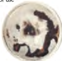
Mold covers the control sample completely
