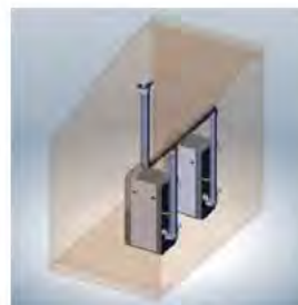
Common vertical vent/ room air
