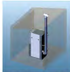
Vertical vent/room air
