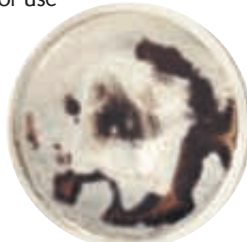
Mold covers the control sample completely
