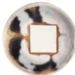
Mold growth is inhibited on the Foster® 40-20™ coating
