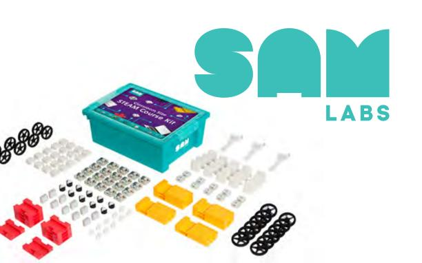
SAM Labs are easy and engaging app-enabled, programmable blocks consisting of inputs and outputs that each have a function of their own. By connecting the physical blocks to the SAM Space app or Google's Workbench, every block sequence can accomplish a new solution - press a button to turn on a light, or use a light sensor to activate an alarm. Take learning further by integrating micro:bit with SAM Labs in the new Learn to Code Kits.
