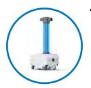
**RoverUV** - The only fully autonomous disinfection robot manufactured in the USA. Powered by 1200 watts of UV-C light, it kills 99.99% of COVID-19 pathogens and is capable of disinfecting over 16,000 square feet on a single charge. Ideal for disinfecting large rooms and spaces, its innovative safety features ensure the robot closes down instantly if it senses any movement within 50 feet.
